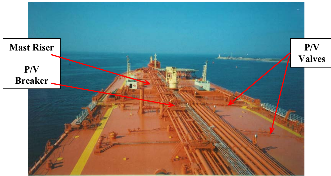
Figure 2.2 – Main Cargo Deck of a Crude Oil Tanker
